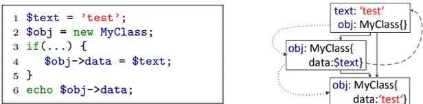
Figure 1: The code on the left creates a new object and assigns data to a property. The corresponding control flow graph is illustrated on the right. The created object `obj` is propagated forward throughout the CFG (dotted arrow). Assigned data to an object’s property is resolved by backwards-directed data flow analysis (dashed arrow).
